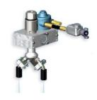
The SG-60 & SG-70 also feature powered rotation, but at much slower speeds. The two options are 10rpm -50 rpm, and 80rpm-500 rpm. Slower rotation speeds increase dwell time and depth of penetration which has been proven to aid removal of thick deposits, particularly at long standoff distances. The SG-E60 is air-powered and the SG-E70 uses a hydraulic motor.
